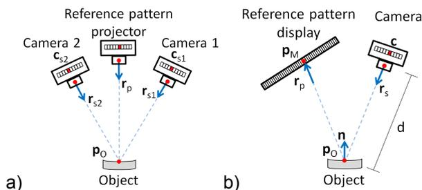
**Fig. 1:** Principles of geometric-optical phase measurement techniques: a) Fringe Projection (FP); b) Phase Measuring Deflectometry (PMD)
