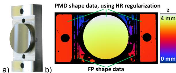
Fig. 2: a) Object surface with locally varying surface roughness; b) PMD shape data, using HR regularization; c) Combined shape data from FP and PMD (using HR regularization) measurements, with invalid areas shown in black and colour-coded height (measurement field size:  $40 \times 20 \text{ mm}^2$ ).
