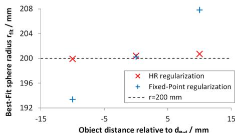
Fig. 3: Radius of best-fit sphere calculated from shape data of spherical mirror (radius of curvature  $r = 200 \text{ mm}$ ) with combined HR test system using HR-Regularization and Fixed-Point Regularization with constant  $d_E$  (see section 2), for different relative object positions  $z$ .
